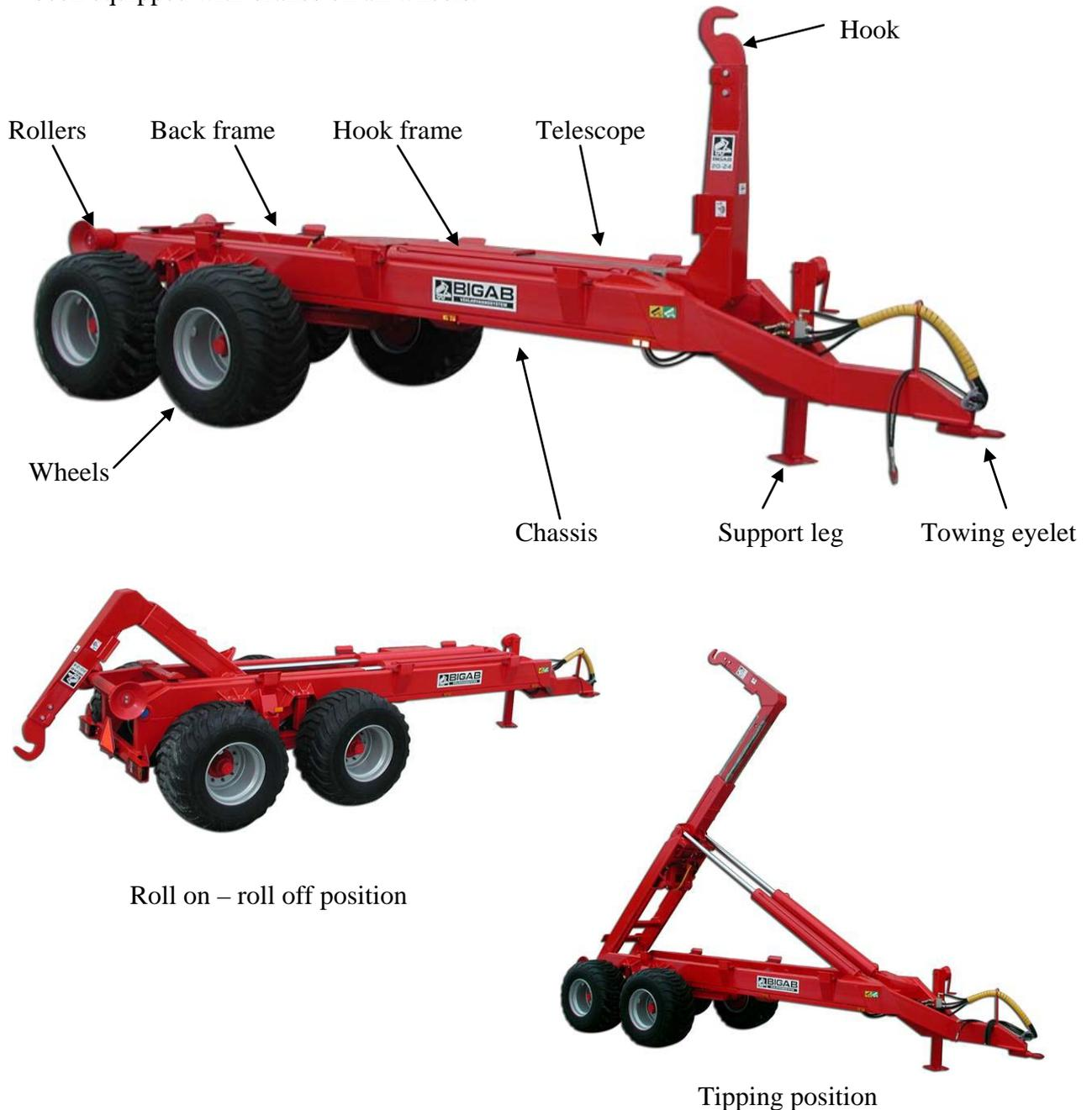
*Figure 1. Design of the device*
