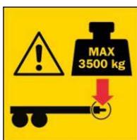
Figure 26. Max. pressure on towing eyelet
